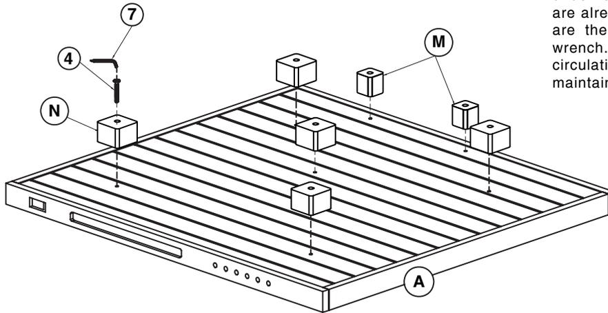
The first step to installing your new sauna will be to insert the legs underneath the floor panel. The holes are already pre-drilled so all you need are the bolts (No. 4) and the Allen wrench. This is necessary to allow air circulation to flow underneath and maintain the integrity of the unit.
