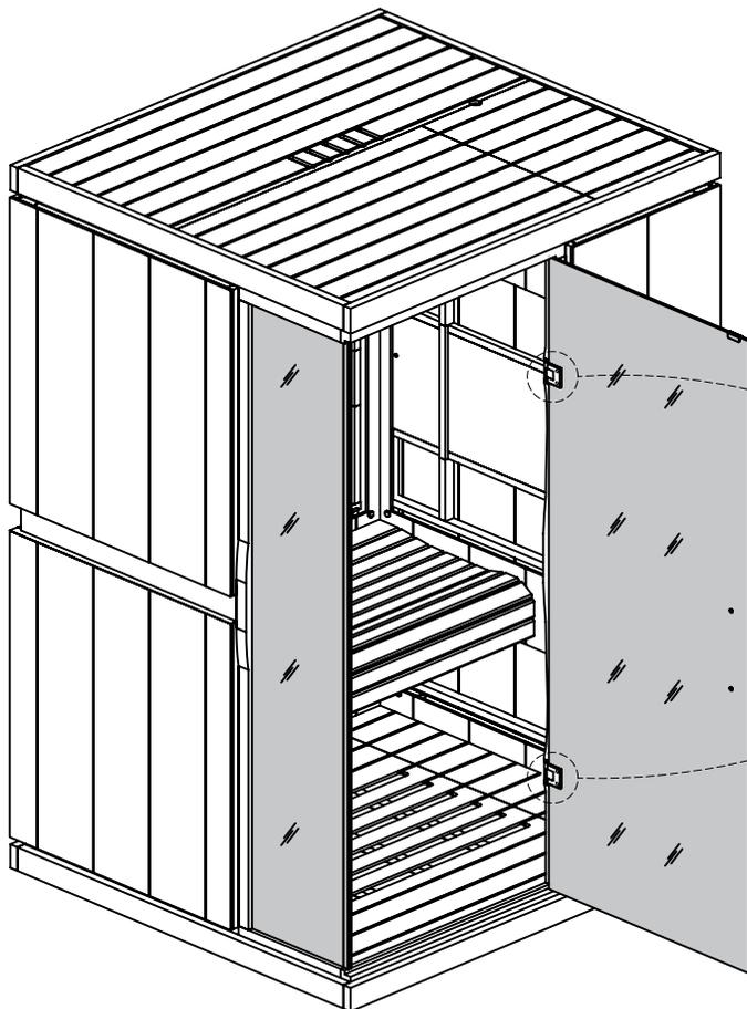
Using the Allen wrench, you will tighten the bolts into the hinges as the door is inserted. Make sure the bolt is inserted firmly. Each hinge will have four plastic gaskets. The door will be inserted between the four gaskets.
