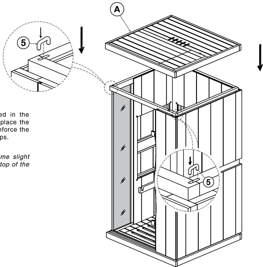
After all four U-clips are inserted in the corners, the next step will be to place the roof on top. The roof will also reinforce the walls in position along with the clips.
