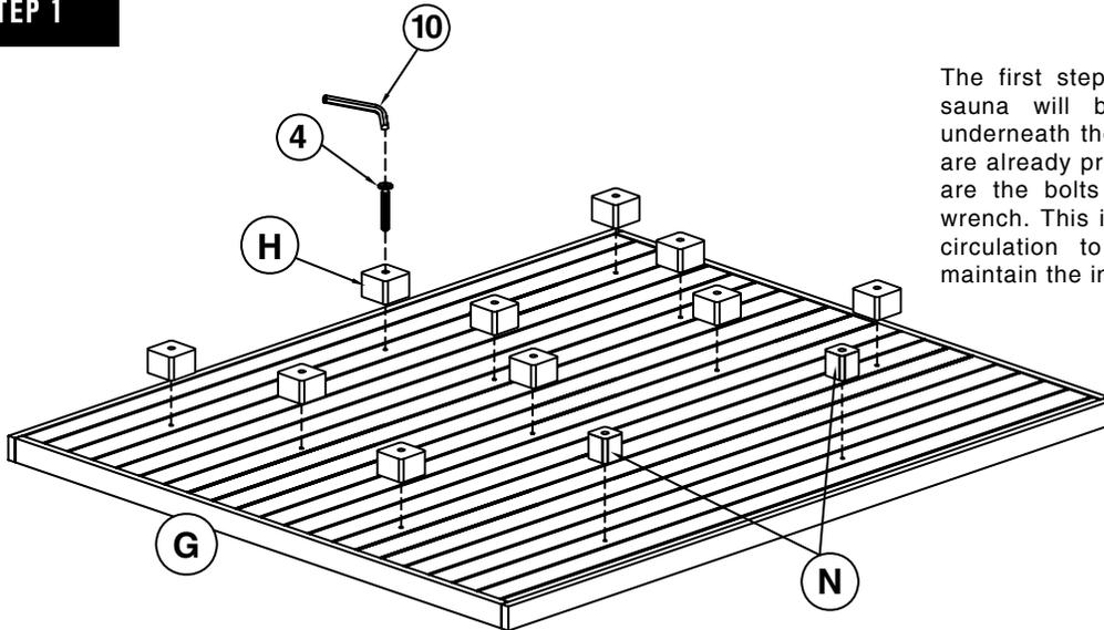
The first step to installing your new sauna will be to insert the legs underneath the floor panel. The holes are already pre-drilled so all you need are the bolts (No. 4) and the Allen wrench. This is necessary to allow air circulation to flow underneath and maintain the integrity of the unit.
